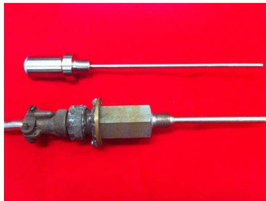
Figure 3. Air Temperature (PRT) probes (top) slim current (bottom) thick previous.
