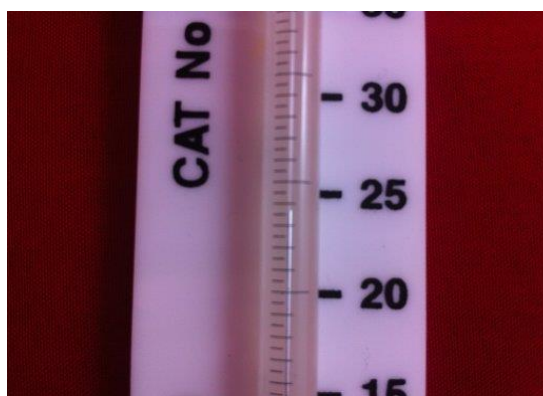
Figure 2. Ordinary dry bulb thermometer with a temperature measurement of 23.7 °C.
